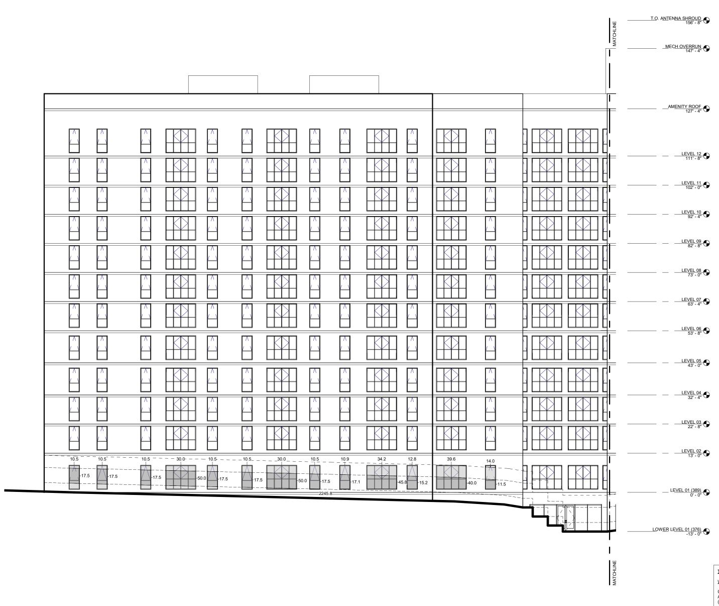
TRANSPARENCY CALCULATIONS: WEST ELEVATION (PARTIAL) - COX AVENUE GROUND LEVEL SURFACE AREA: (WITHIN 0'-0" - 12'-0") 2,246 SF AREA OF REQ'D TRANSPARENCY FOR RESIDENTIAL (NONE REQ'D PER UDO SECTION 1.59): NR ACTUAL AREA OF TRANSPARENCY WITHIN 0'-0" - 12'-0" PROVIDED: 569 SF (25%) ACTUAL AREA OF TRANSPARENCY WITHIN 3'-0" - 8'-0" PROVIDED: 317 SF
