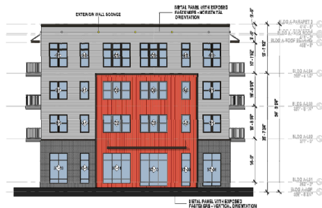
ELEVATION - BUILDING A WEST 3/8" = 1'-0"
