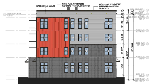
ELEVATION - BUILDING B NORTH 1 88'0" x 11'0"
