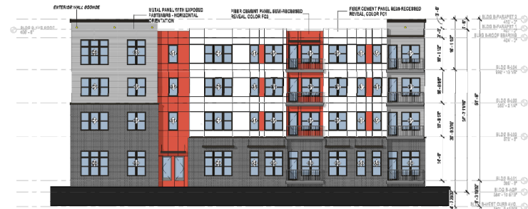
ELEVATION - BUILDING B WEST 4 88'0" x 11'0"
