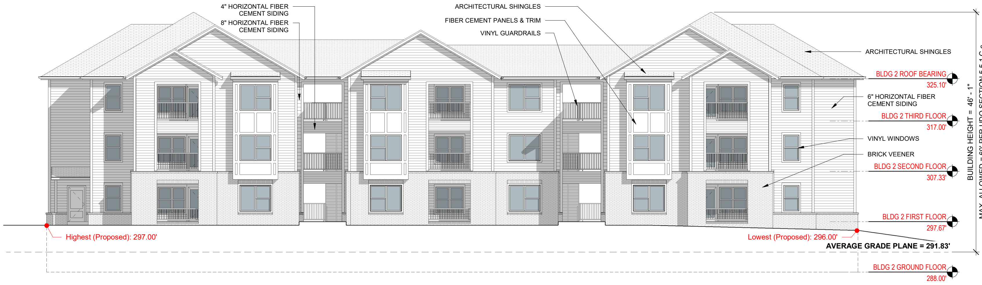
BUILDING 2 - WEST ELEVATION PRIMARY STREET FRONT PLANE [1] 3/32" = 1' - 0"
