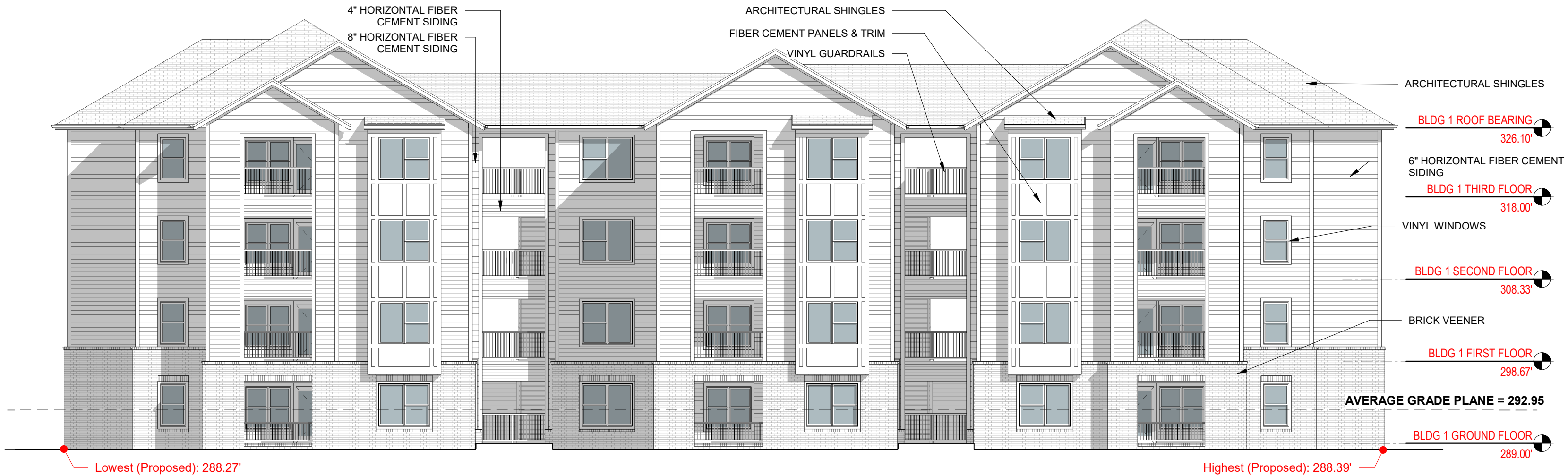
BUILDING 1 - EAST ELEVATION REAR PLANE [4] 3/32" = 1' - 0"
