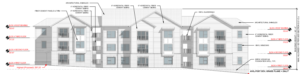
BUILDING 4 - SOUTH ELEVATION PRIMARY STREET FRONT PLANE [1] 3/32" = 1' - 0"
