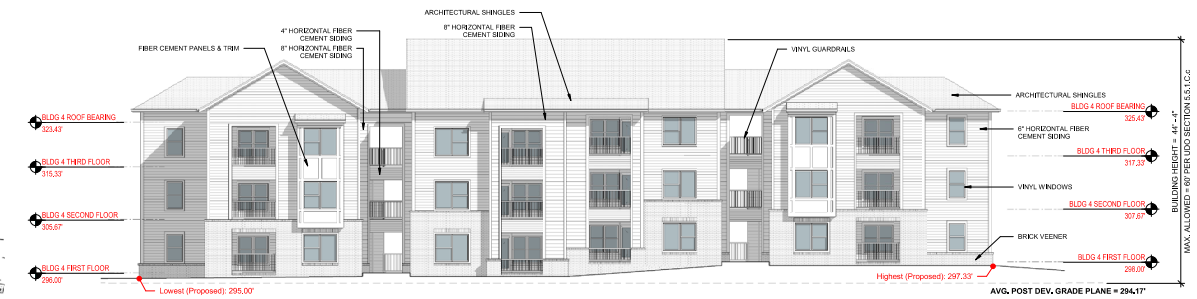
BUILDING 4 - NORTH ELEVATION REAR PLANE [4] 3/32" = 1' - 0"
