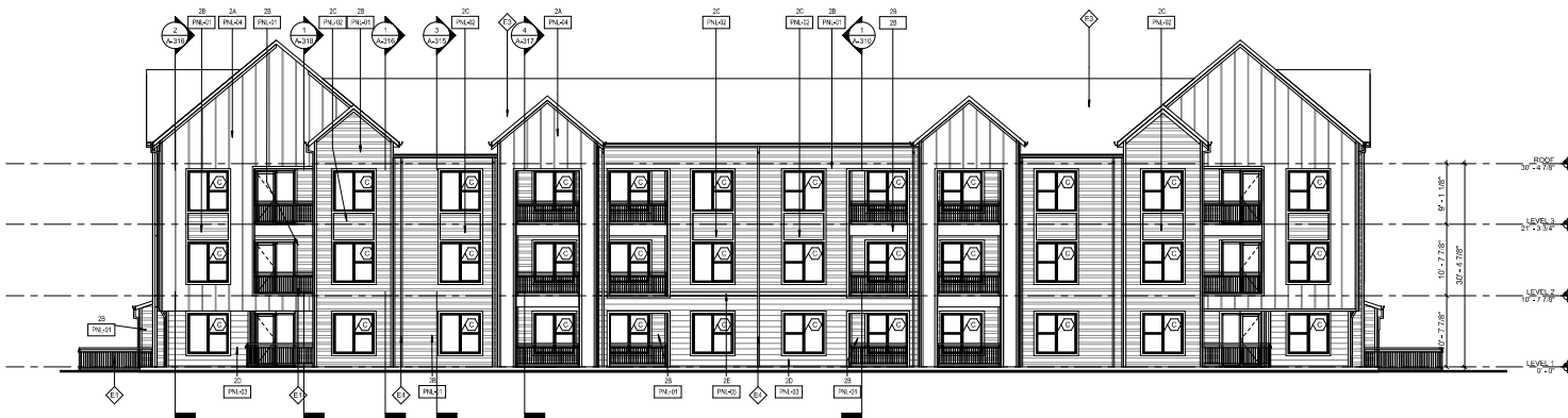
BUILDING B - REAR ELEVATION - BLD 1 1/8" = 1'-0"
