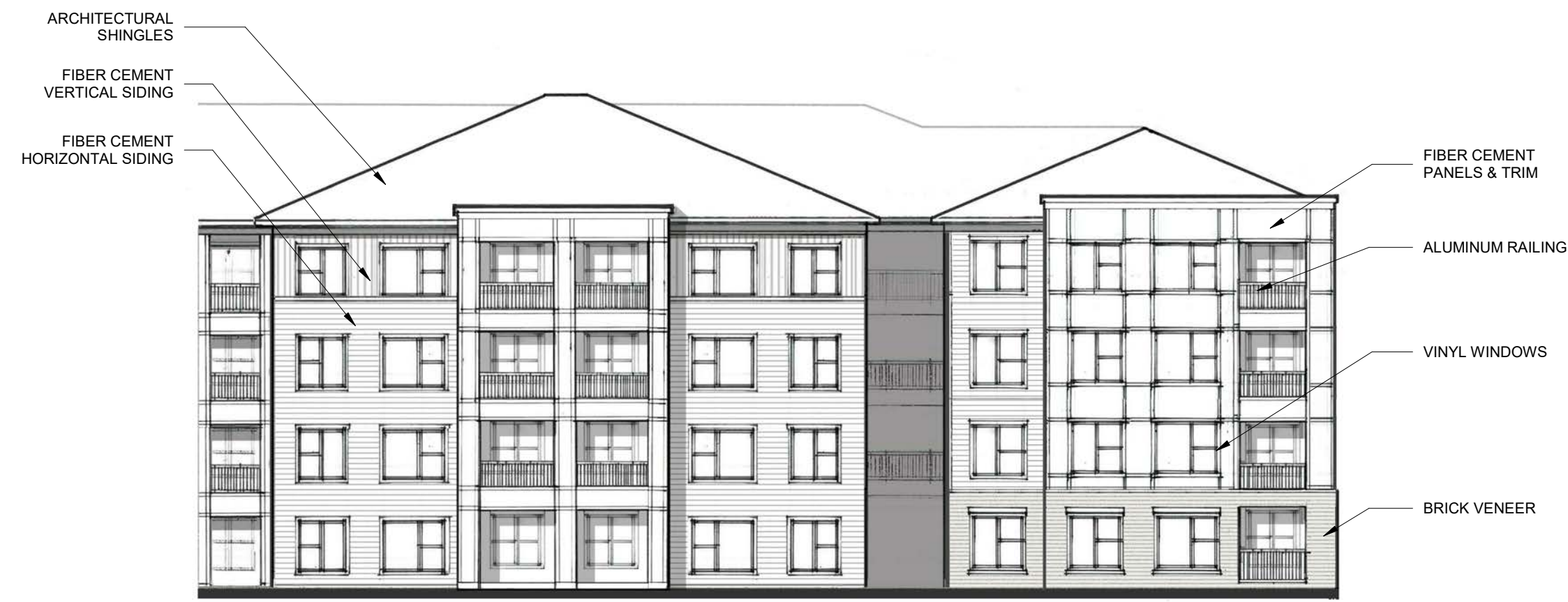
COURTYARD WEST ELEVATION
