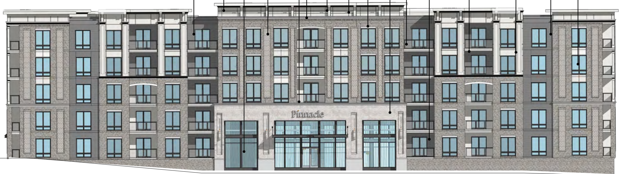
Elevation - Building 1000 East Side Scale: 1/8" = 1'-0"
