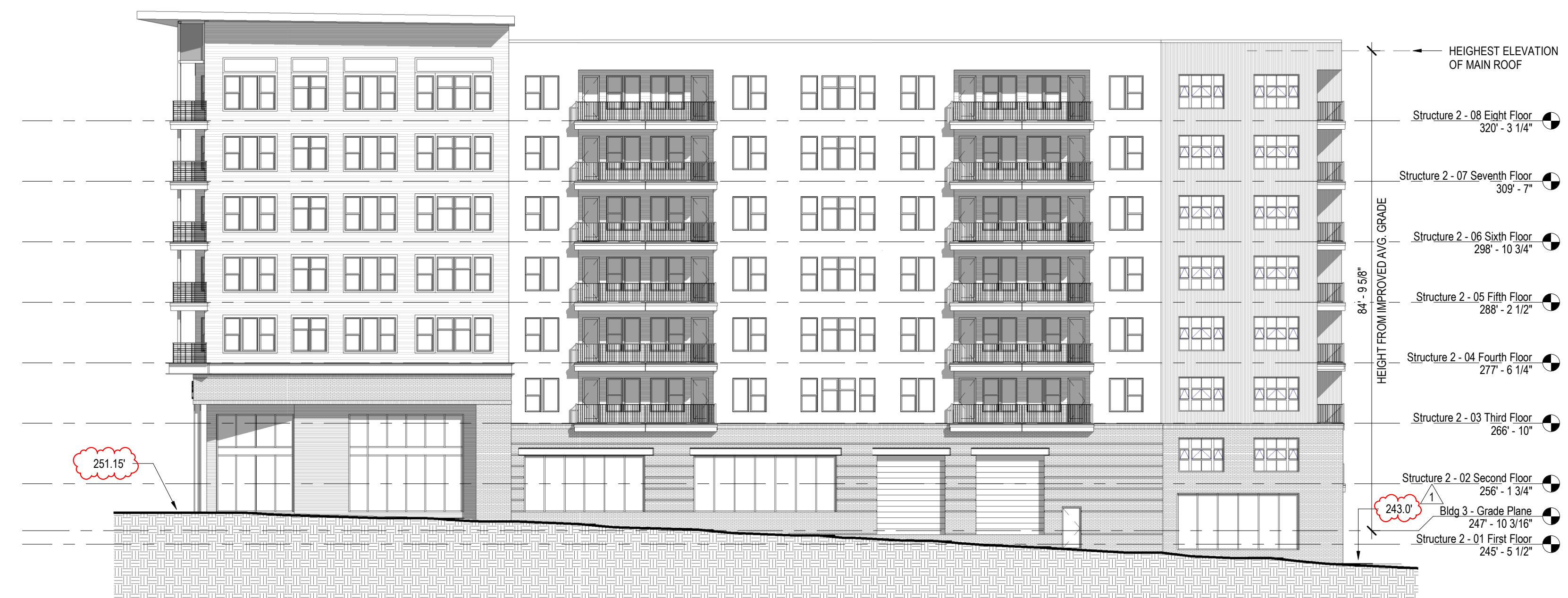
BUILDING 3 NORTH ELEVATION
