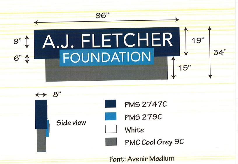
Construction: Fabricated aluminum panel with aluminum dimensional letters. Not internally illuminated.
