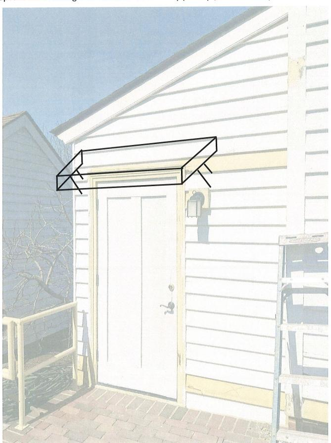
Will be wood-framed with angled brackets attaching back to structure. Beaded edge on brackets to match handrails at front porch. Roof finish to be architectural shingle to match existing roof. Painted to match house. Anticipate relo-
