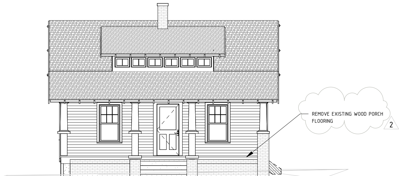
1 FRONT ELEVATION - DEMOLITION SCALE: 1/8" = 1'-0"
