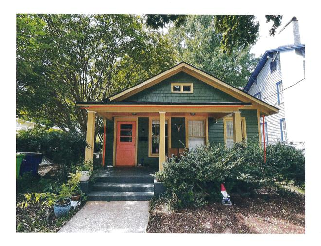
The gutters will be installed along the length of the house, one on either side of the roof, with one along the front of the porch. Downspouts will be along the front left porch column, and along the front left and right side of the house. It will drain towards the street.
