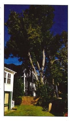
smaller, this location did not present an issue; but now, the tree has grown significantly and the gradual expansion of the basal area (or root crown) of the tree has pushed the surrounding soil away and against the retaining wall such that the wall is now leaning significantly. Note in the picture (at right) that "vertical" is demonstrated by viewing the corner of the yellow structure in the background. The pecan tree is on the left of the wall.
