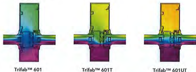
Thermal simulations showing temperature variations from exterior/cold side to interior/warm side.
