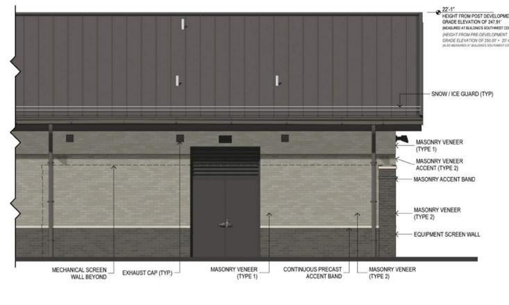
**G11** WEST BUILDING ELEVATION (INSIDE SCREEN WALL)
