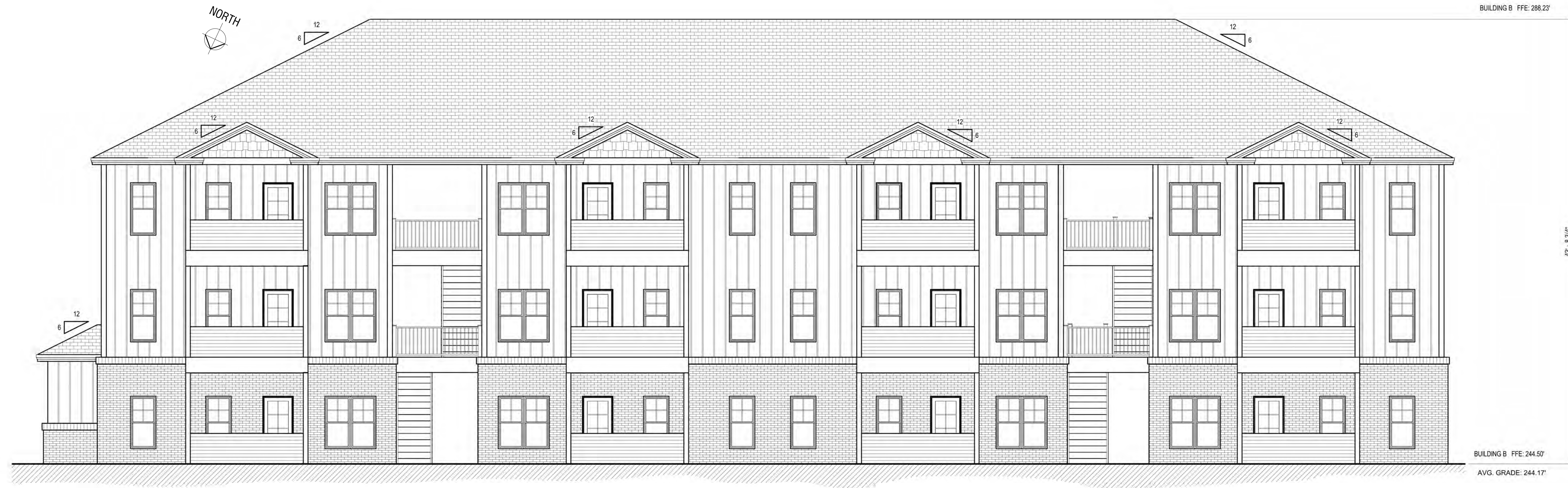
1 FRONT ELEVATION SCALE: 3/16" = 1'-0" BUILDING B: (244.50' + 243.83') / 2 = 244.17'
