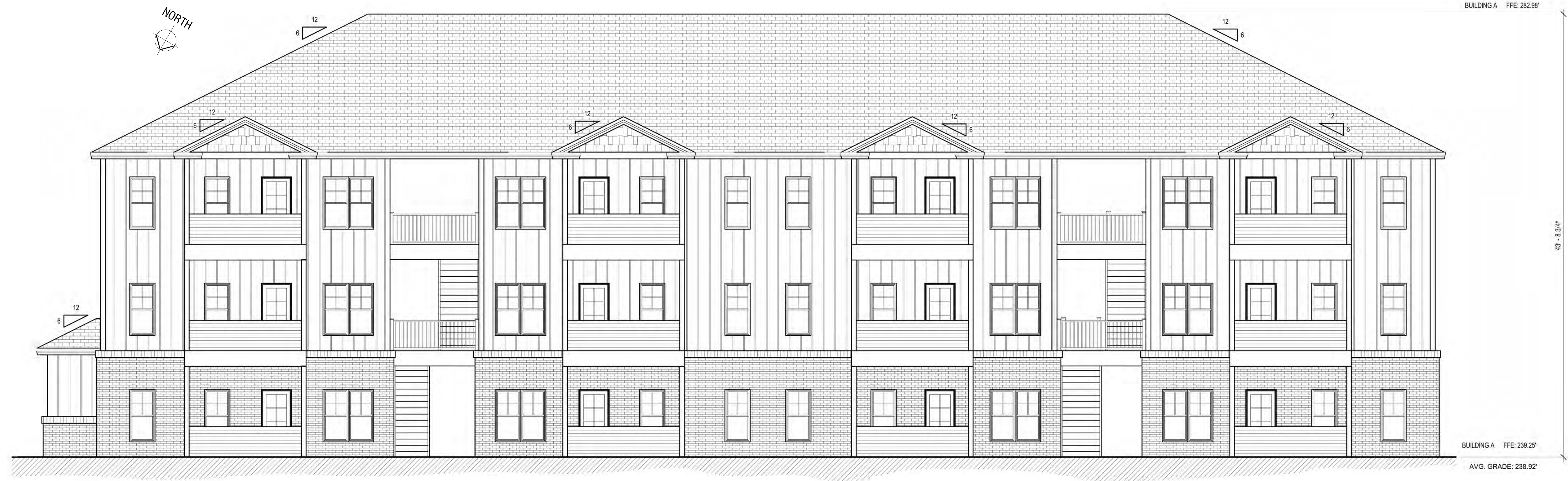
1 FRONT ELEVATION SCALE: 3/16" = 1'-0" BUILDING A: (239.25' + 238.58') / 2 = 238.92'
