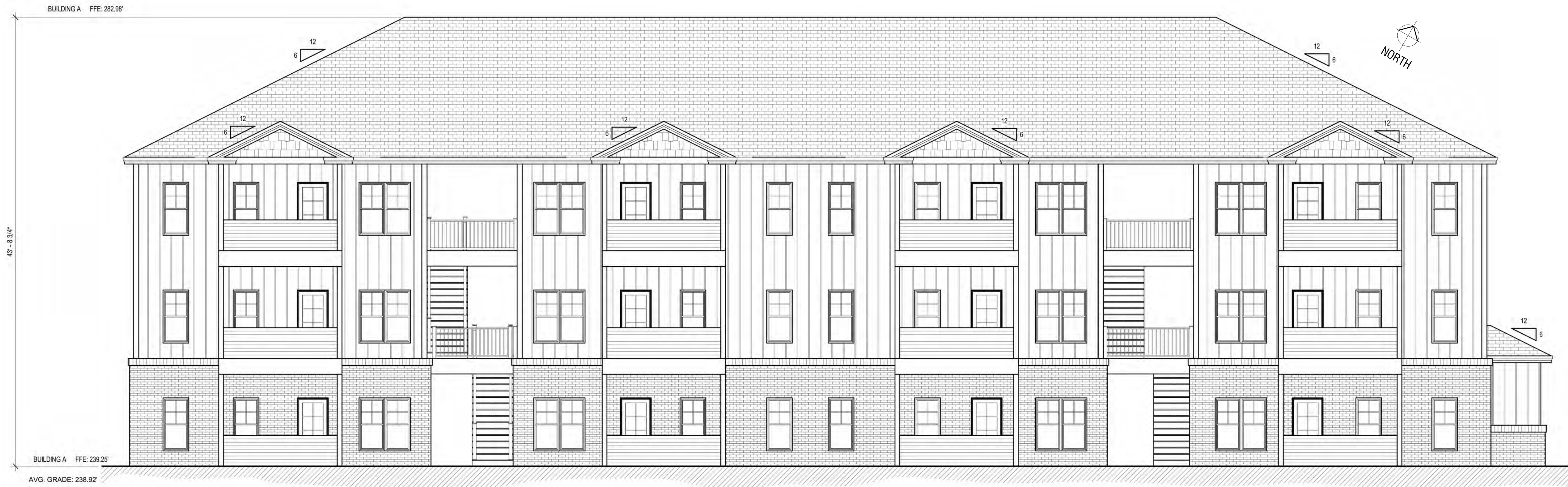
1 REAR ELEVATION SCALE: 3/16" = 1'-0" BUILDING A: (239.25' + 238.58') / 2 = 238.92'
