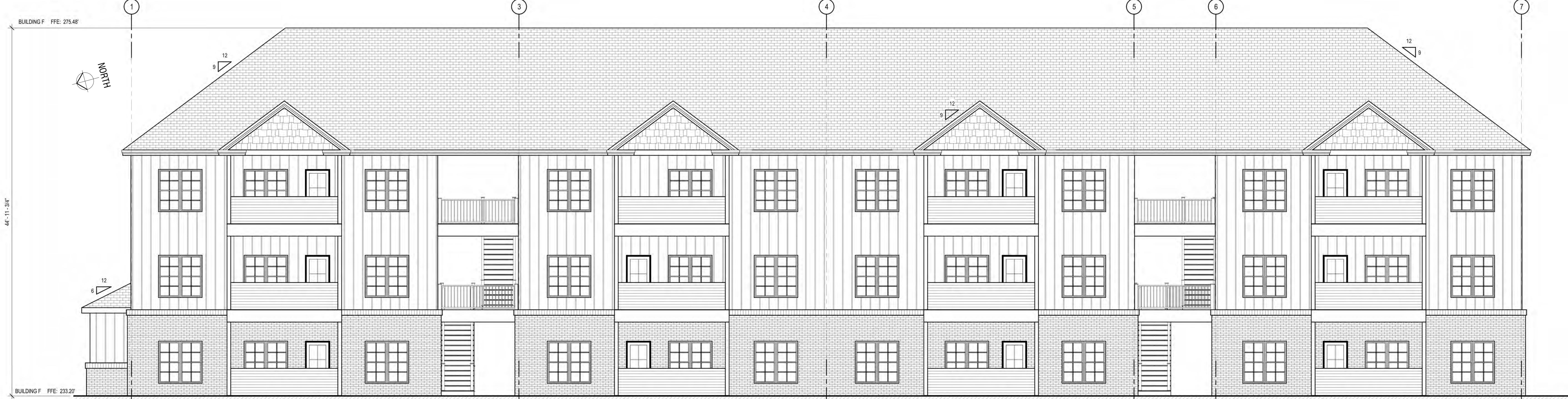
1 FRONT ELEVATION SCALE: 3/16" = 1'-0" BUILDING F: (233.20' + 233.20') / 2 = 233.20'
