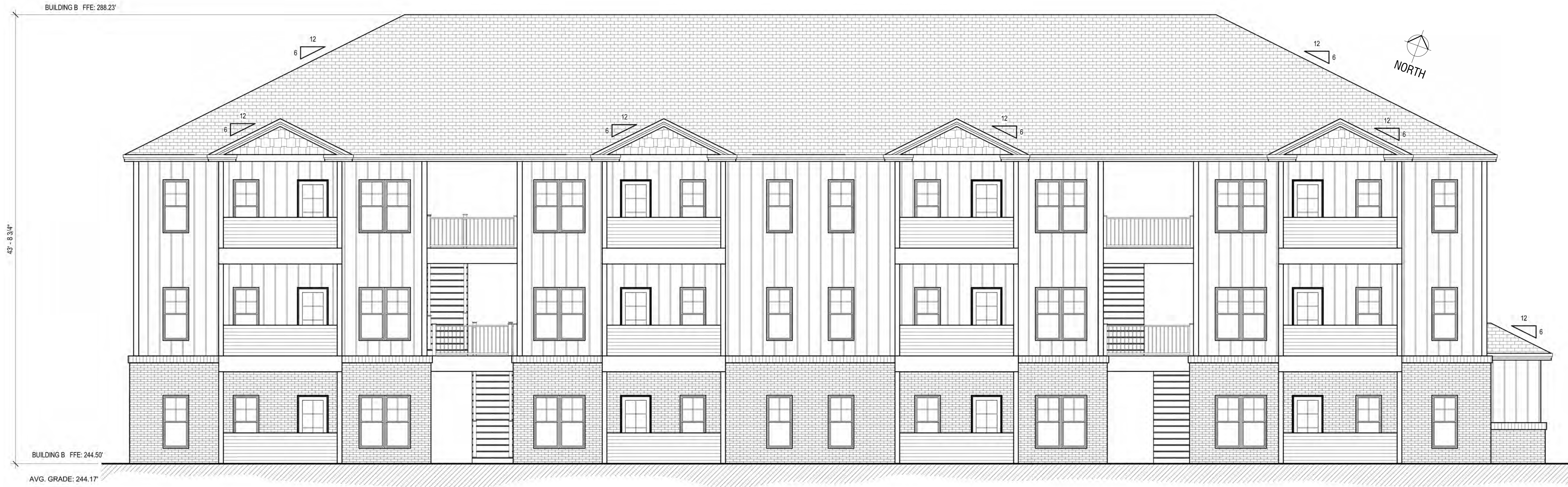
1 REAR ELEVATION SCALE: 3/16" = 1'-0" BUILDING B: (244.50' + 243.83') / 2 = 244.17'
