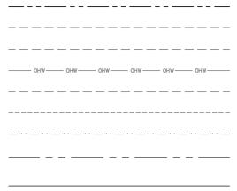
EXISTING PROPERTY LINE EXISTING ABUTTING PROPERTY LINE EXISTING RIGHT-OF-WAY EXISTING OVERHEAD POWER LINE EXISTING ABUTTING PROPERTY LINE EXISTING EDGE OF PAVEMENT EXISTING EASEMENT PROPOSED CITY OF RALEIGH GENERAL UTILITY EASEMENT PROPOSED LOT LINE
