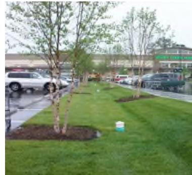
**Figure 3** Bioretention in Commercial Development
