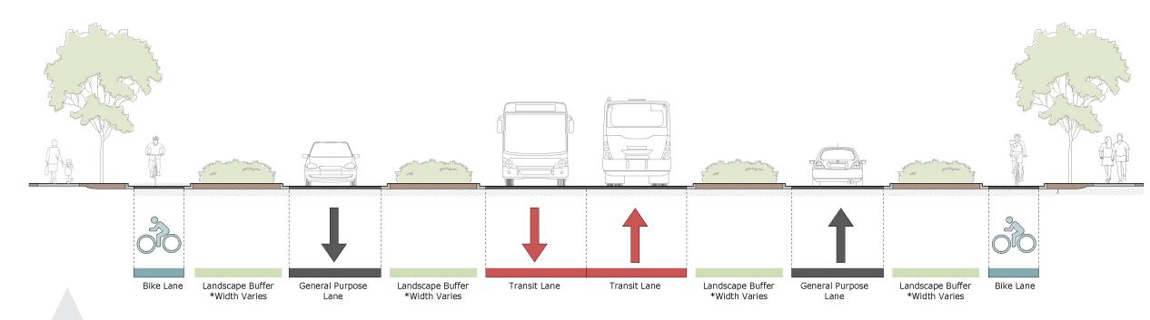
**Bus-Only Lane:** a median or center lane for BRT vehicles separated from general traffic.
