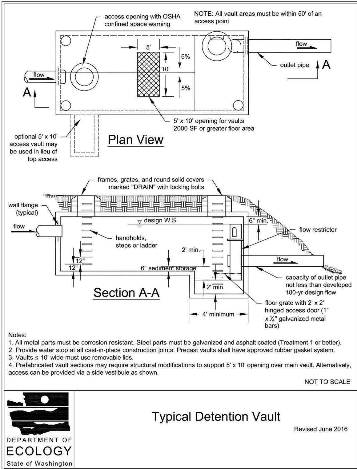
**Figure 5.6.3 Example Schematic of an Underground Detention System (Source: Washington Department of Ecology, 2019)**
