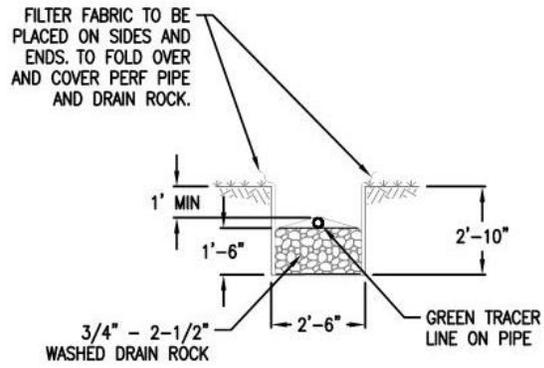
LINE TRENCH SIDES WITH PERMEABLE FILTER FABRIC AS SHOWN, ADD 18" OF DRAIN ROCK. PLACE PERF. PIPE AND COVER ALL.
