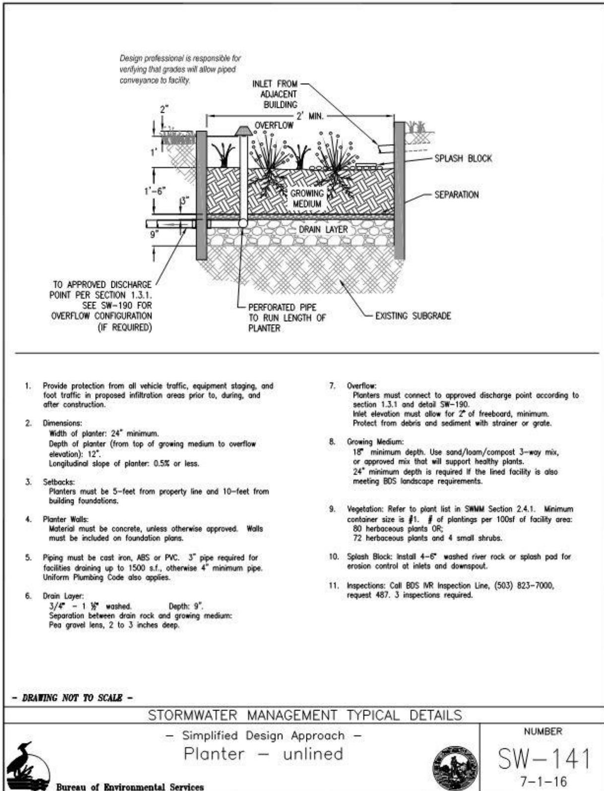
**Figure 5.6.2.b Example Construction Detail of a Planter (Unlined)**
