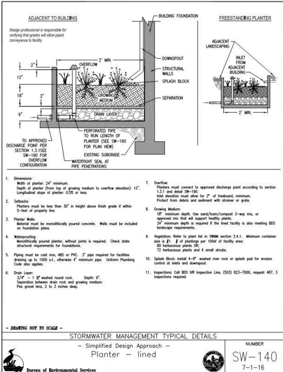
Figure 5.6.2.a Example Construction Detail of a Planter (Lined)
