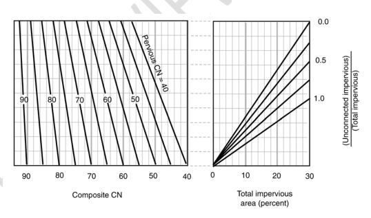
Figure 3.6.4.2.b <u>Composite CN With Unconnected Impervious Area (Total</u> <u>Impervious Area Less than 30%)</u>
