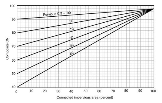
Figure 3.6.4.2.a Composite CN with Connected Impervious Area
