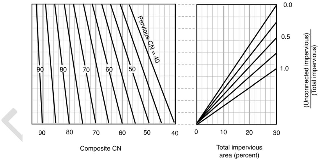
Figure 3.6.4.2.b Composite CN With Unconnected Impervious Area (Total Impervious Area Less than 30%)
