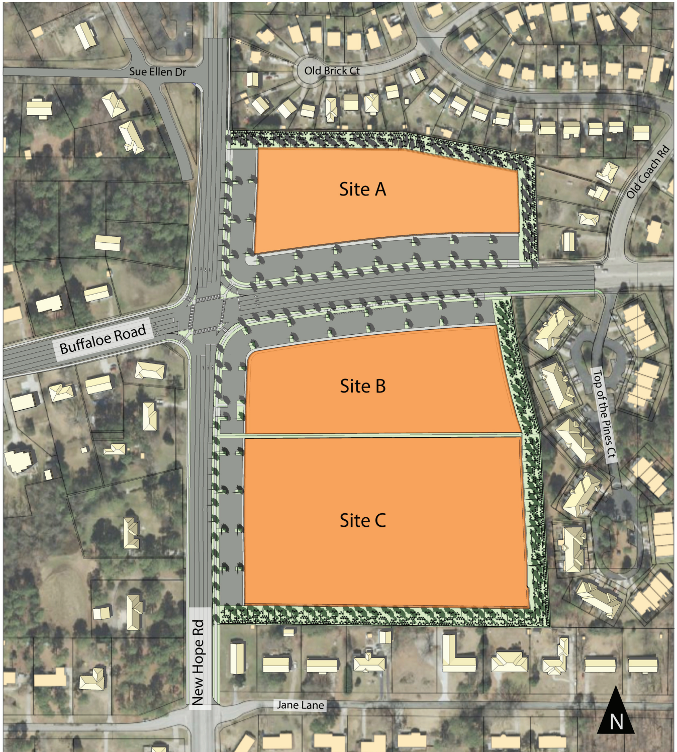
Figure A-1. Intersection with basic Parking Limited frontage standards and transitional buffer with Type 3 (Wide) protective yard
