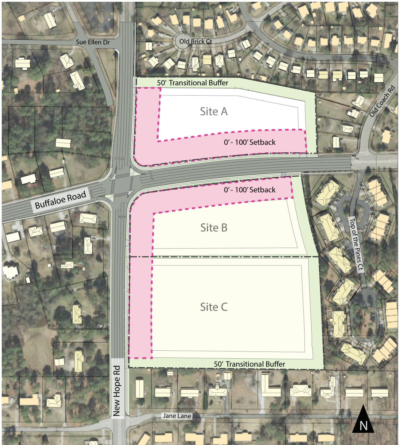
Figure A-2. Parking Limited build-to area (50% of the building width would have to be within 0' - 100' of the primary street; 25% of the building width would have to be within 0' - 100' of the side street).
