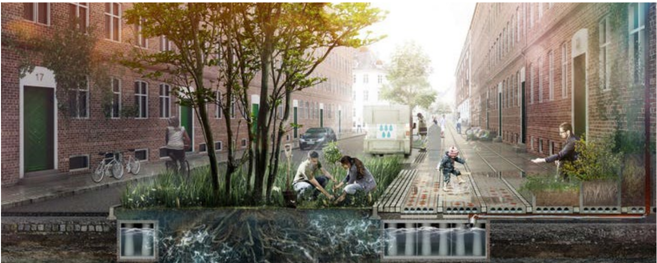
▲ Climate Tile Project in Copenhagen, DK. An example of how streets or "green fingers" that abut a floodplain area can incorporate permeable surfaces that capture/filter excess water and help naturally recharge aquifers. http://theconversation.com
