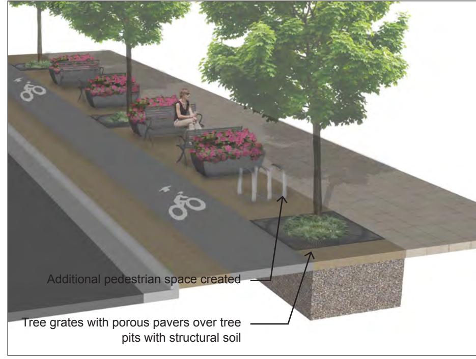
Streetscape with trees in tree pits planted in structural soil and permeable pavers above. This configuration provides maximum space for street furnishings, seating areas, etc.
