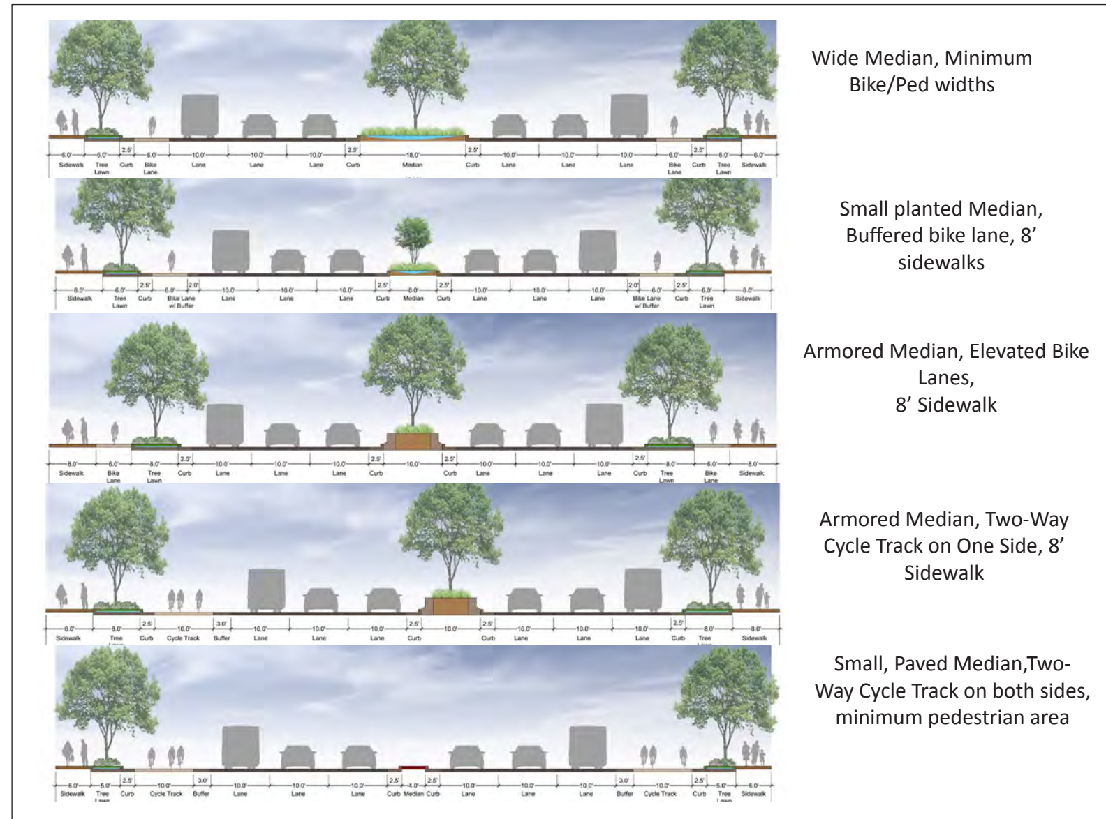
The Design and Planning team worked with stakeholders and the Community to develop and compare multiple configurations of streetscape cross-sections. Trade-offs between bike, pedestrian, planting, and vehicular spaces were explored and prioritized.
