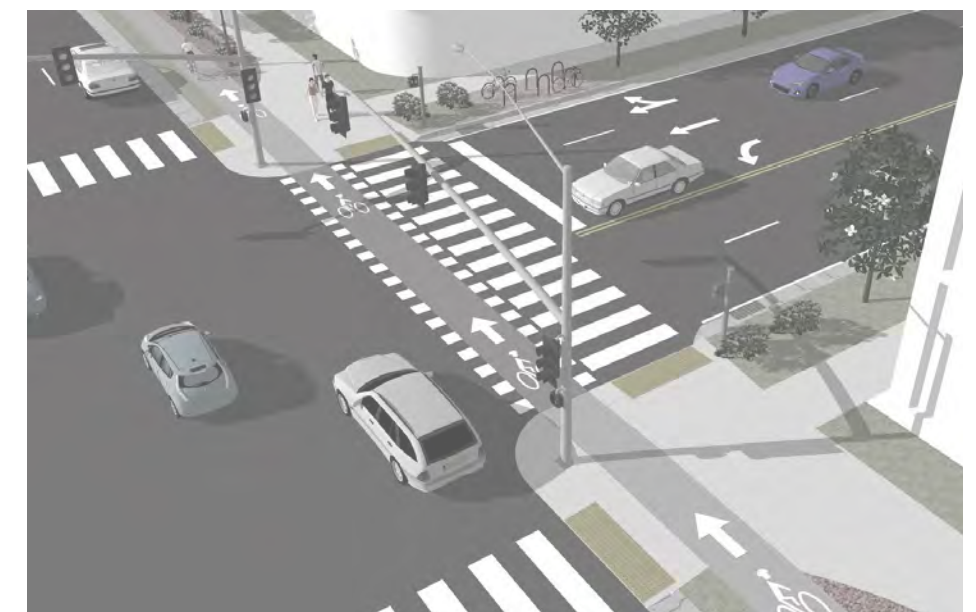
SIGNALIZED INTERSECTION TREATMENT
