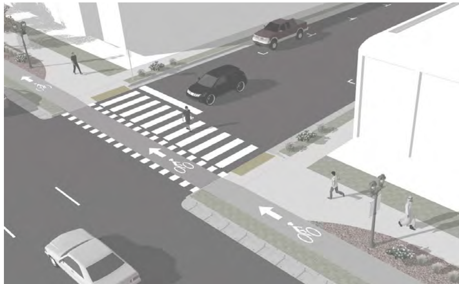
MINOR UNSIGNALIZED INTERSECTION TREATMENT
