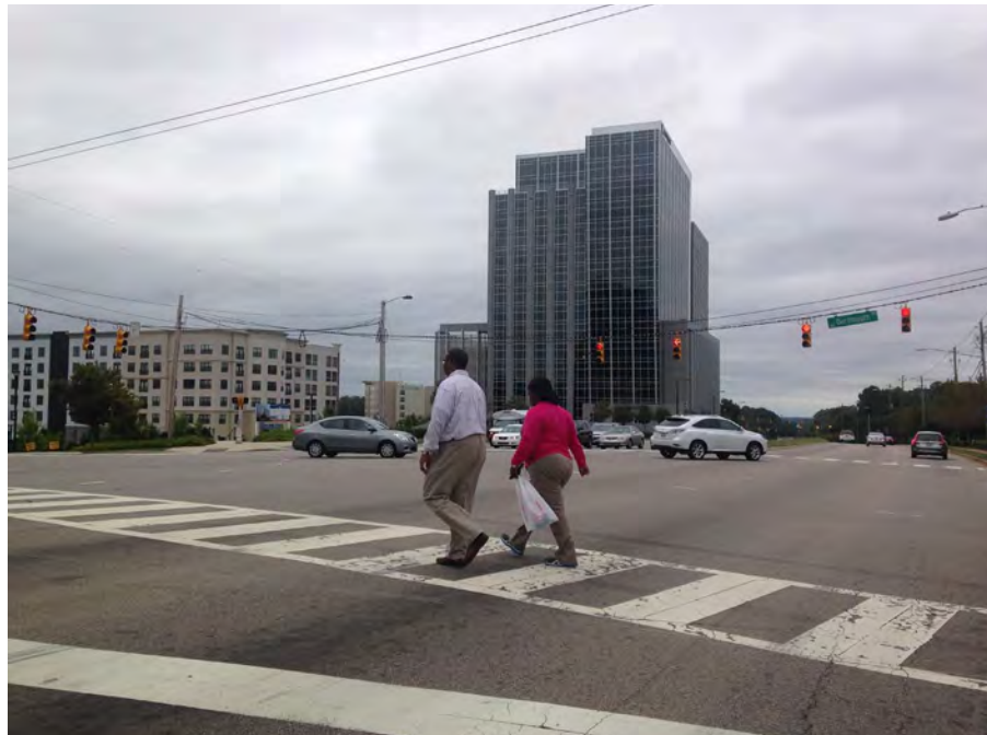
In recently developed North Hills area many of the crosswalks are high visibility and have pedestrian countdown signals. While these intersections are above average compared to other intersections in the corridor, there is still an opportunity to create pedestrian refuges and a cohesive streetscape that promotes walkability.
