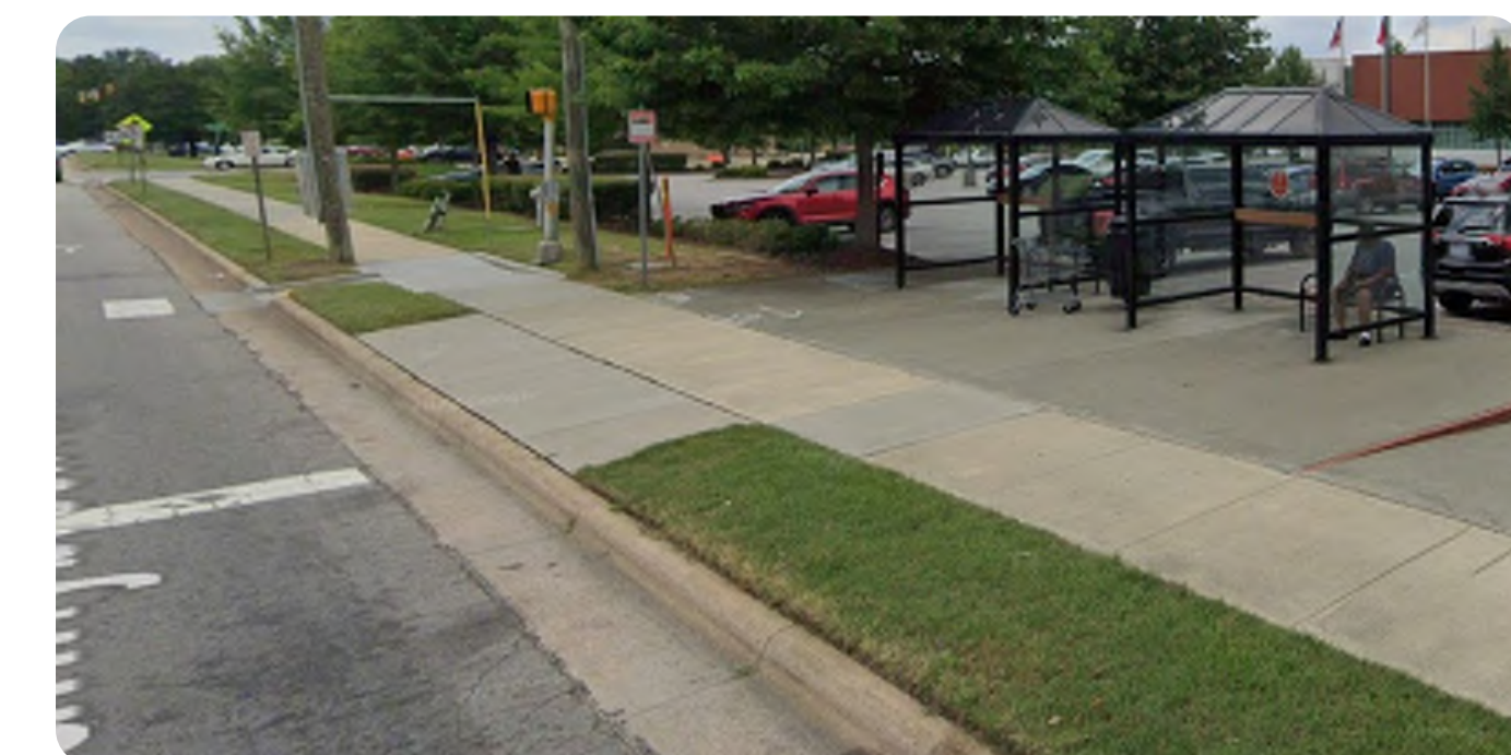
EXAMPLE ADA LANDING PAD - 30' IN LENGTH
