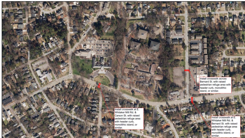
Oaks at Whitaker Glen - Roadway Work
