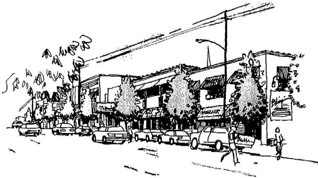
FIGURE 2. STREETScape WITH CONSOLIDATING AND STRAIGHTENING OF LINES AND POLES
