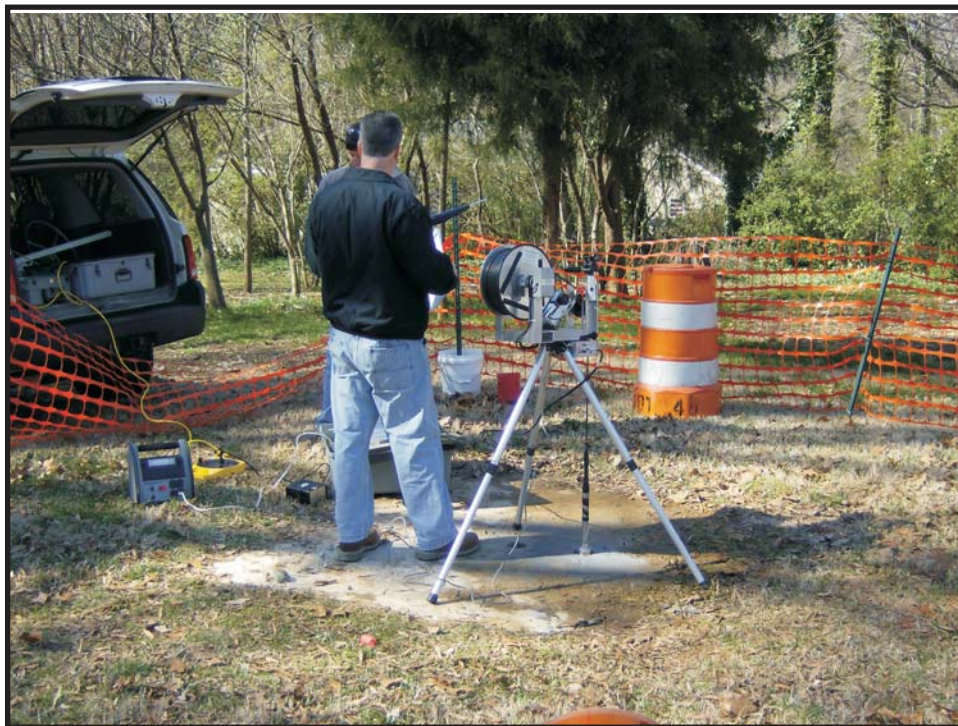
Camera being lowered through cap into well shaft.
