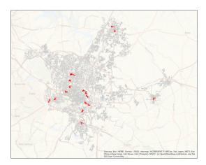
Further analysis refined the probability of failure results, identifying clusters of similar high-risk pipe segments to help Raleigh Water build more efficient asset management plans now and in the future..
