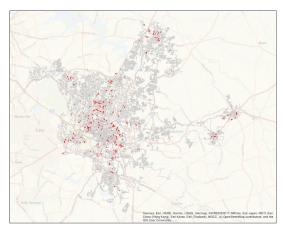
Xylem's solution identified the top 1% of at-risk pipeline segments based on their probability of failure. These assets are scattered throughout the city.
