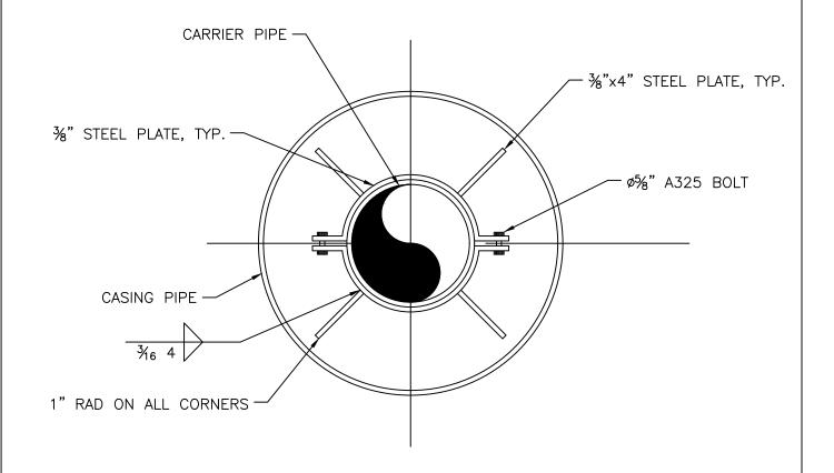
NOTE: USE A MINIMUM OF TWO SPIDERS PER PIPE JOINT ONE FOURTH OF THE PIPE JOINT LENGTH IN FROM BOTH THE BELL AND SPIGOT ENDS.
