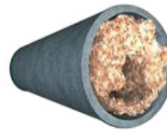
Fully clogged service
