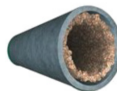
Partially clogged service
