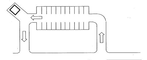
A-4. Where a circular through movement is not possible, maneuvering space in front of any dumpster as noted in C-1 below must be provided (30' min.). Backup and turnaround space must be in an aisle with a minimum width of 16' and a depth of 30', and min. inside curb radius of 30'.
