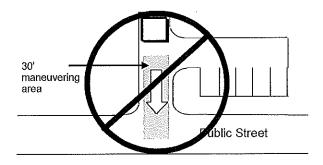
A-3. Parking areas must allow for a circular through movement wherever possible to avoid back-up movements.
