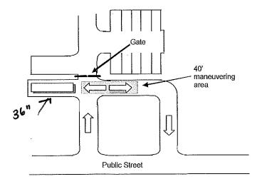
A-6. Alleys used for solid waste collection vehicles that serve individual residential units must be a min. 16' in width. Inside curb radii must be min. 30'. All alleys to be traversed by solid waste collection vehicles must meet the residential street standard of 6" sub-base and 2.5" asphalt surface course.
