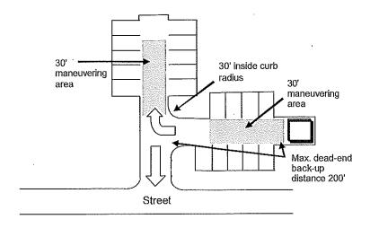
A-5. Access to roll-off collection devices as noted in C-1 below shall provide 40 feet of clear maneuvering area from the end of the compactor. Access to roll-off device shall not be restricted by any private gate or door, except in accordance with C-5 below, and must meet the standards of A-2 above.
