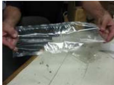
**OEP plastic air bladder used in damper/diffuser**
