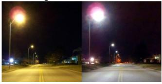
The City's LED Streetlight Pilot Project replaced traditional street lighting with high-efficiency LED lights. After a successful pilot, Raleigh began replacing 30,000 conventional lights in fall 2015. It is estimated that LED streetlights operating up to 12 hours a day should last a minimum of 15 to 20 years. These lights use far less energy than traditional lights. They can be recognized by their brighter white light.
