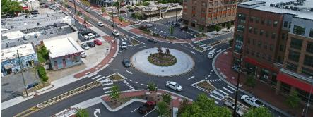
Roundabouts are a roadway formation. They are typically used to slow traffic speeds and reduce accidents. They also keep traffic moving and reduce stops and starts from traffic lights, which reduces vehicle travel times, reduces greenhouse gas emissions, and increases air quality.
