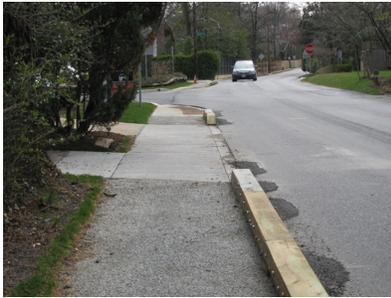
Photo 34. View of crushed stone sidewalk with timber curb.
