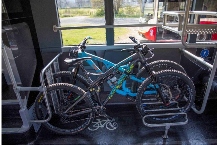
Figure 7.2 On-Board Bike Storage 25
