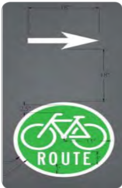
St. Louis, MO is currently studying the impact of a small bike wayfinding medallion pavement marking.
